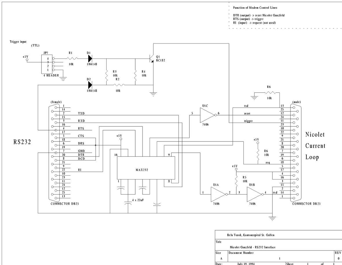
Figure 2. Circuit diagram of the RS232 – Nicolet current-loop interface.
