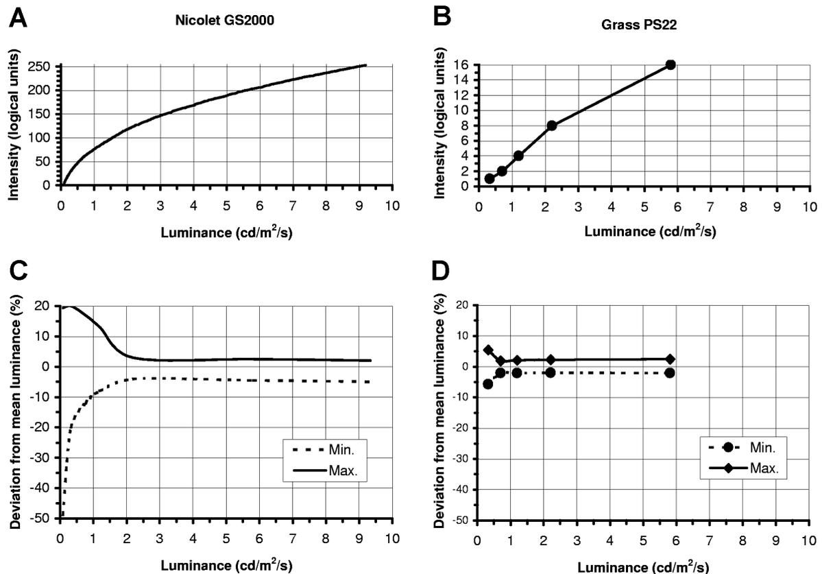
Figure 3. Flash intensity measured at all programmable intensity levels (without filters) of the Nicolet GS2000 stimulator (A) and the Grass PS22 photostimulator (B). Maximal and minimal deviation from the mean intensity in % of the Nicolet (C) and the Grass photostimulator (D).
